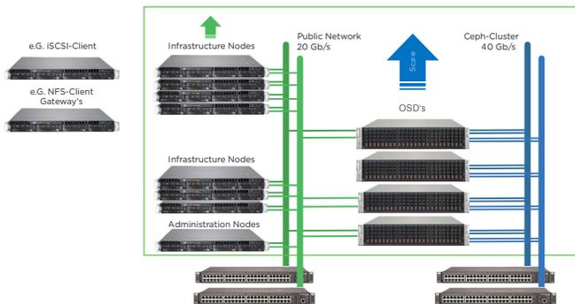
Figure 2: Set-up of an SES Cluster
