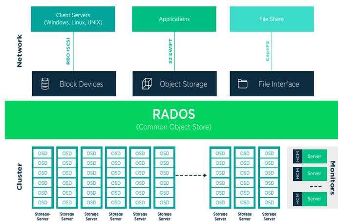
Figure 1: Architecture of Ceph/SUSE Enterprise Storage
