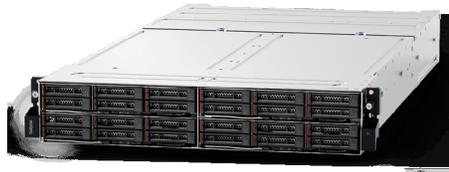
**ThinkSystem SD530**—This ultradense two-unit, four-node platform delivers more compute power in less space and supports the use of GPUs for diverse workload requirements.
