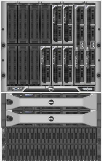
The M1000e chassis, with the half height M620s, and full height M820s.
