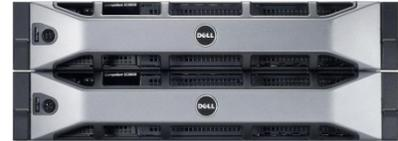
The system then uses a series of drive shelves, with you basing your drive choice off both your capacity and IOPS requirements. In this example we show a shelf of 24 300GB/15,000rpm drives. Alternative configurations, including all flash-based storage, are also available.
