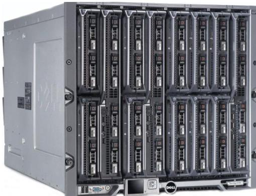
The chassis can contain up to 16 M620 half-height servers, or up to eight M820 full height servers, or a mix of the two.
