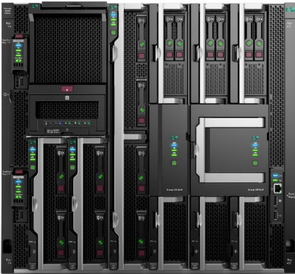
**Figure 2.** HPE Synergy frame—front view
