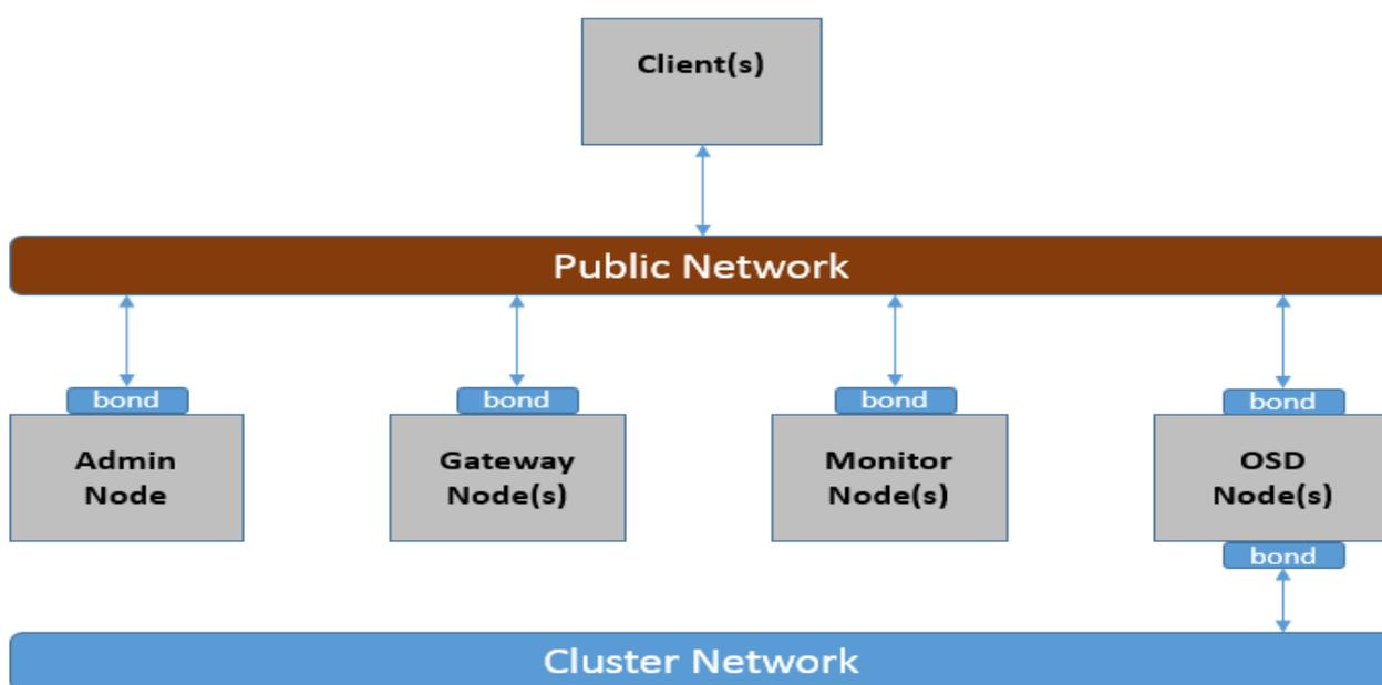
Figure 2. Sample networking diagram for Ceph cluster
