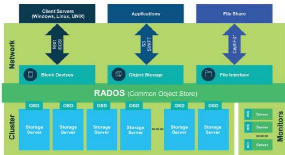
Figure 1. Ceph architecture diagram
